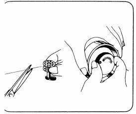
Take off bobbin from spindle and cut thread.
